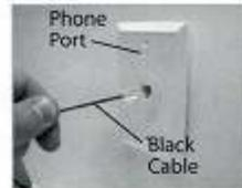
**Step 14** Make sure **All Devices** with the same phone number as your DSL Line have Phone Filters. This includes telephones, fax machines, caller ID boxes, satellite TV receivers, TiVo devices, and answering machines.
