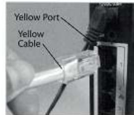
**Step 9** Make sure that your computer is turned on. Then, plug the other end of the **Yellow Cable** in the **Ethernet Port** on the back of the computer.
